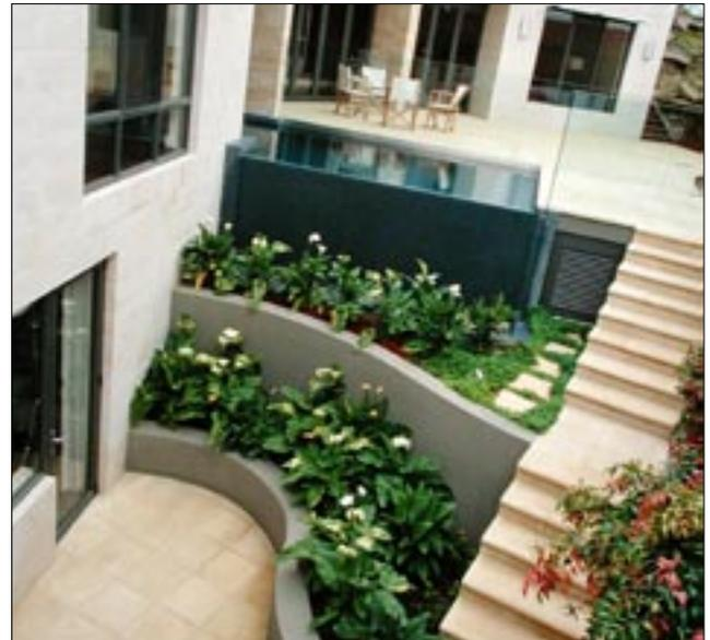
**The small pool** was included in the main courtyard area so that it would be easily seen and therefore used a lot. The glass pool fence not only provides the required safety in a visually minimal way; it also assists in moderating the north-east breezes in this outside area. The 'wet-edge' effect helps to provide evaporative cooling to the lower courtyard, which has less access to cooling breezes. [\[See: Passive Cooling\]](#)
