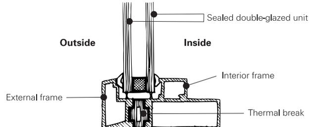
**A thermal break** is often used to reduce the heat conduction of aluminium frames. A thermal break splits the frame components into exterior and interior pieces using a less conductive material to join them.
