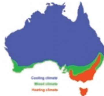
**Cooling (or tropical, subtropical and hot arid) climates** are warmer climates where most energy is used to cool the home. Geographically, most of Australia has a cooling climate. In these climates windows should be designed to keep the heat outside. [See: [Glazing – Hot Humid](#)]
