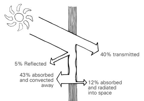
**Reflective glass** has either a vacuum-deposited metal coating or a pyrolytic coating. Vacuum-deposited coatings are soft and must be glazed facing indoors. Pyrolytic coatings are hard and durable and can be glazed facing outdoors. Where glare may annoy neighbours, reflectivity should be kept below 15 to 20 percent.
