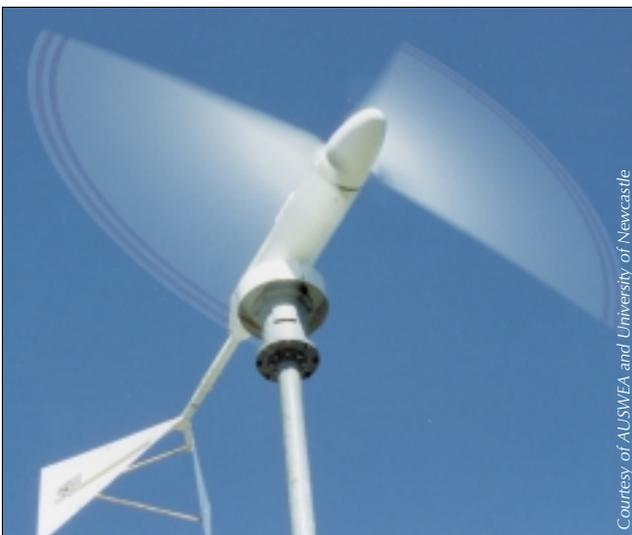
**The main body of the wind generator** comprises a set of blades, the alternator and the tail section. The power of the wind makes the blades turn. The blades are connected to the rotor inside the alternator which turns and generates electrical power. The tail ensures that the wind generator is facing directly into the wind.
