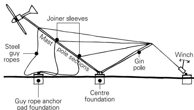
**The typical tower** is designed so that it can be lowered and raised by tilting the tower with a gin pole and winch.
