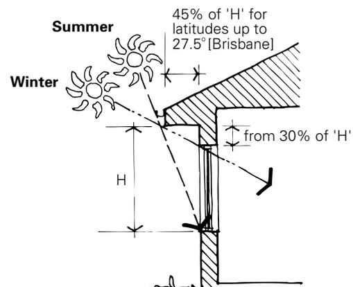
**The general 'rule of thumb'** for calculating eaves width is given above. This rule applies to all latitudes south of and including 27.5°S (Brisbane, Geraldton). Within this range the rule is self adjusting - going south winter sun angles decrease, but at the same time the need for solar access increases as climates becomes cooler.
