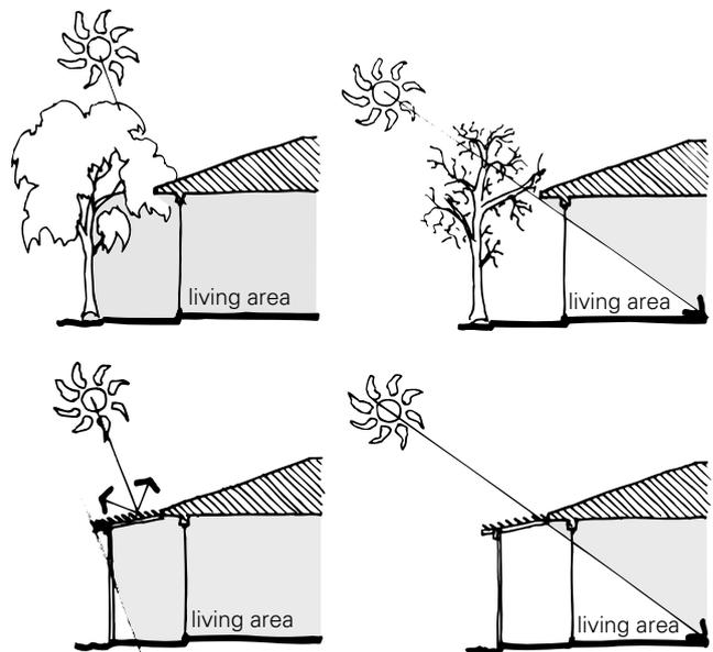
With ideal north orientation sun can be excluded in summer and admitted in winter using simple horizontal devices, including eaves. For situations where ideal orientation cannot be achieved (eg existing house, challenging site) it is still possible to find effective shading solutions. [See: [Passive Solar Heating; Orientation](#)]
