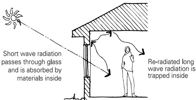
**Heat is gained** when short wave radiation passes through glass, where it is absorbed by building elements and furnishings and re-radiated as longwave radiation. Longwave radiation cannot pass back through glass as easily.
