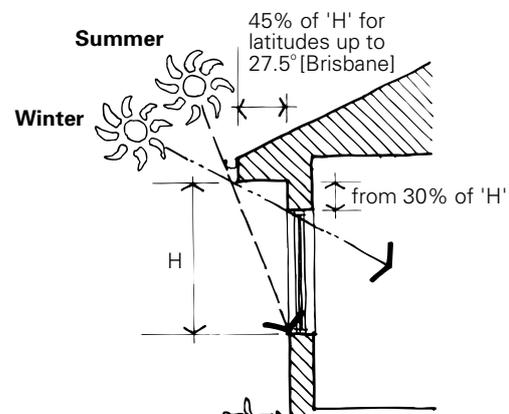
**Permanently shaded glass** at the top of the window is a significant source of heat loss. To avoid this, the distance between the top of glazing and eaves underside should be 50% of overhang or 30% of window height.
