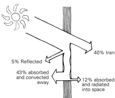
**Heat is lost** through glass by conduction, particularly at night. Conductive loss can be controlled by window insulation treatments such as close fitting heavy drapes with snug pelmets, double glazing and other advanced glazing technology.
