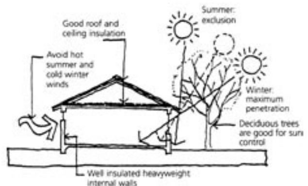
**Heat is re-radiated and distributed** to where it is needed. Direct re-radiation is the most effective means. Design floor plans to ensure that the most important rooms (usually day-use living areas) face north for the best solar access. Heat is also conducted through building materials and distributed by air movement.
