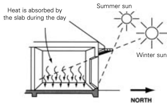
**Adequate levels** of exposed (ie. not covered with insulative materials such as carpet) internal thermal mass in combination with other passive design elements will ensure that temperatures remain comfortable all night (and successive sunless days). This is due to a property known as thermal lag.
