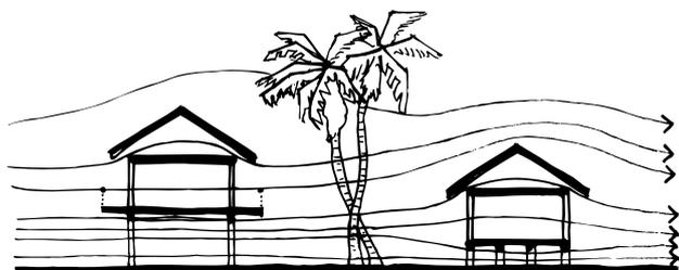
**Design** narrow, elongated building forms for best performance, with the long elevations opening up to cooling breezes. Elevating the house so that air can circulate beneath it will also assist performance.
