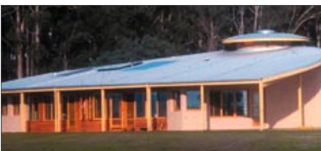
The house itself is completely self contained and autonomous. It has a grid connected solar array, captures rainwater for drinking, and treats wastewater for irrigation on-site. There are two sheds (used for woodworking and as an artist's studio) and a large garage.
