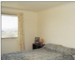
**Cross ventilation** was improved by adding a second window to the main bedroom to draw cooling breezes across the bed. The two room depth plan otherwise provided good cross ventilation to the living areas. [\[See: Passive Cooling\]](#)
