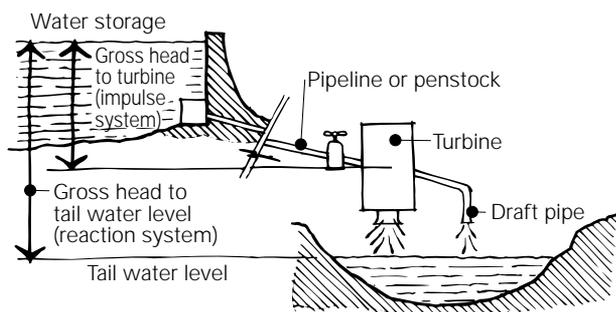
Depending on the type of turbine, the water may be discharged direct to the tail water or through a pipe.
