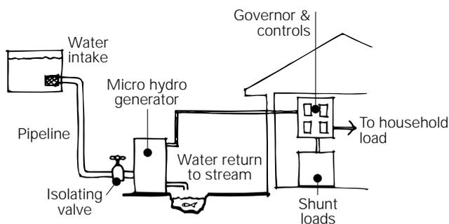
In micro hydro systems water turns a wheel or a runner (like a propeller) to rotate a turbine and produce electricity. The wheels come in different shapes and sizes depending on the site and the type of turbine.
