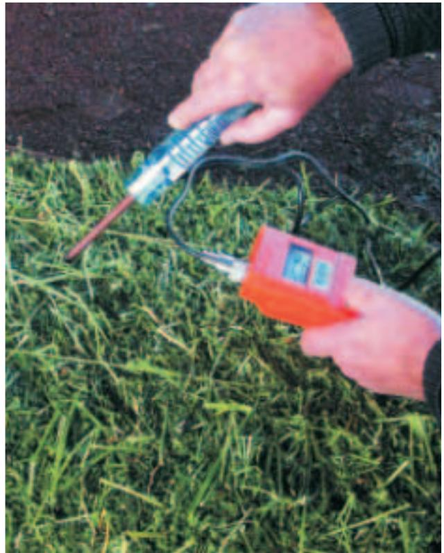
**Using a moisture meter to check the moisture content of hay about to be stored**
