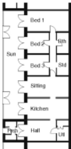
**Each home is comprised of six bays** 3 metres wide by 6 metres deep. The roof slopes from front to rear, so that on the south side (the front), the bay is 3 metres high and slopes down to about 2.3 metres high at the rear. In the front wall of each bay is a pair of full length glazed doors, with a window above, forming a large glazed opening for solar access.
