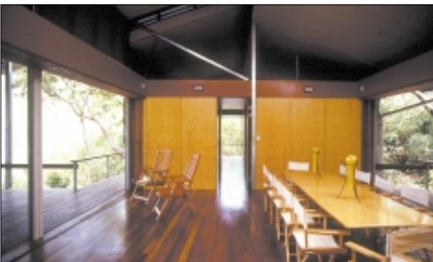
The house was designed to be built from modular components, fabricated off site and transported to site by barge for erection. A 900mm modular design allowed standard material sizes to be used throughout. This reduced costs and minimised wastage in construction. All plywood and aluminium paneling was made to a 900mm wide grid to minimise any waste at the factory and to ensure that there was no site waste generated from construction.
