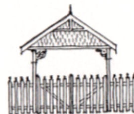
A SIMPLE CAR-PORT OF TIMBER CONSTRUCTION BLENDED WITH A FRONT PICKET FENCE
