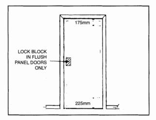
Mark and drill screw holes and screw fix hinges to door.
