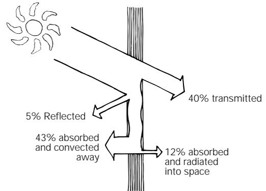
**Solar control glass** reflects some of the sunlight, absorbs some heat, convects most of it away outside and transmits the rest. These windows reduce cooling energy requirements and are rated 2.5 stars by WERS. [See: [How to use WERS](#)]
