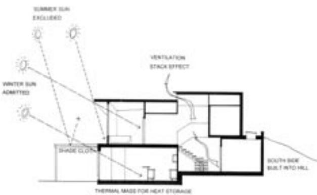
Passive solar design - Cross section
