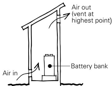
**Ventilation** can be achieved naturally or by installing fans and electrical vents. The amount of ventilation required depends on the number of battery cells and the charging current. A large battery bank using large charging currents needs more ventilation.
