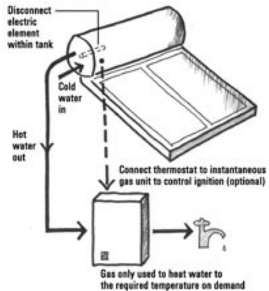
The **electric element has been removed** from the solar hot water service to reduce greenhouse gas emissions. The solar hot water service and the instantaneous gas unit have been connected in series so that gas is only used to boost water temperature when it is actually required. [See: [Hot Water Service; Solar Hot Water](#)]
