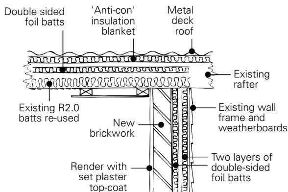
**Two layers** of *Foil Batts* with air gaps between each layer were installed. If the building had sarking (reflective foil laminate) in its original construction, one layer of *Foil Batts* would have been sufficient.
