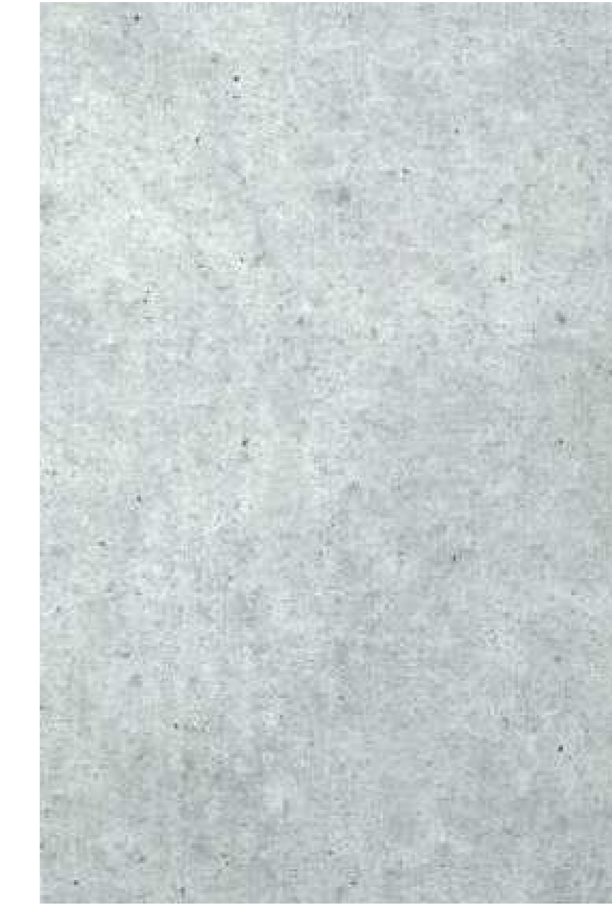
EF03 CONCRETE - OFF FORM FINISH
